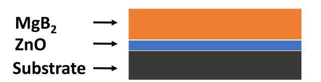
ZnO Buffer thickness  $\rightarrow$  30 - 165 nm MgB<sub>2</sub> thickness  $\rightarrow$  1.0 - 2.0  $\mu$ m
